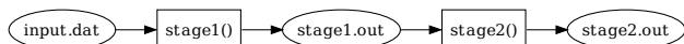
Figure 3: Example Python script that implements a file-based workflow, and accompanying dataflow graph where boxes are code and circles are data files.
