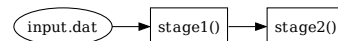
Figure 4: The Python script of Figure 3 refactored to take advantage of IncPy’s automatic memoization. Data flows directly between the two stages without an intermediate data file.
